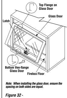
INSTALLING OR REMOVING GLASS DOOR
